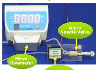
Piezoelectrio Micro Pump The Low Pulsation Micro Pump Module is a module to adjust the flow of a piezoelectric micro pump at the µl/min level using a micro needle valve. In the setup in the left picture, the output flow from the module is being measured by a micro flowmeter. The features of this module make it suitable for various fields, such as flow cytometers, cell culture equipment, etc.
